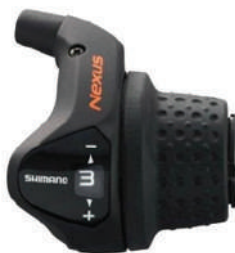
Derailleur A - we change when do not rotate the pedals (crank)
